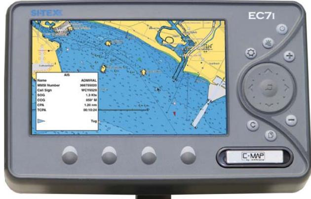
When integrated with compatible AIS products, SI-TEX EC-Series Plotters provide boaters with important information on surrounding vessels equipped with Class A (commercial) and Class B (recreational) AIS transponders. New software enhancements improve the ways boaters can view and use this important information, including how AIS target data is overlaid onto these plotters' C-MAP MAX electronic charts.
